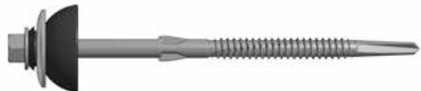
110mm self drilling steel screws for hot rolled steel between 3mm and 6mm - DF12-FCW-5.5 x 60 (80 for vertical).
